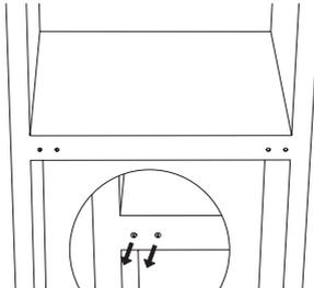
11. Stand up the unit and put the door on the bottom hinge. Make sure the bottom hinge core is inserted in the door hole. Then move the hinge hole cover of bottom door from left side to right side.
