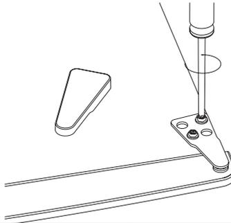
3. Remove the hole cover with a flat screw driver.
