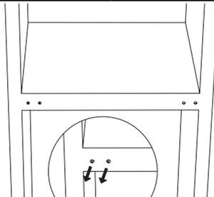
7. Lie down the rear of cabinet on a soft pad. And unscrew the bottom hinge and leveling foot.
