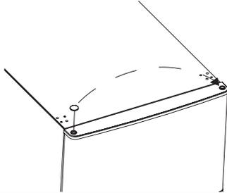
5. Unscrew the middle hinge and then lift the bottom door and put it on a soft pad to avoid scratch.
