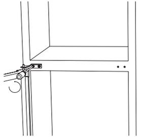
13. Install the upper door with the upper hinge.
