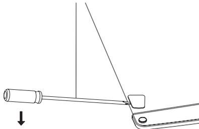
4. Move the core cover from left side to right side. And then lift the upper door and place it on a padded surface to prevent it from scratching.
