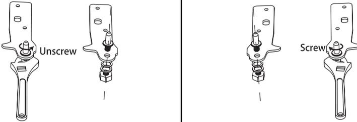
9. Install the hinge at left side and foot base at right side. Then screw two levelling feet with their original parts.
