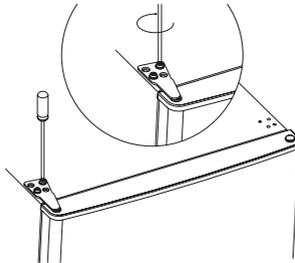
14. Clap in the hinge cover and hole cover on the top of unit.
