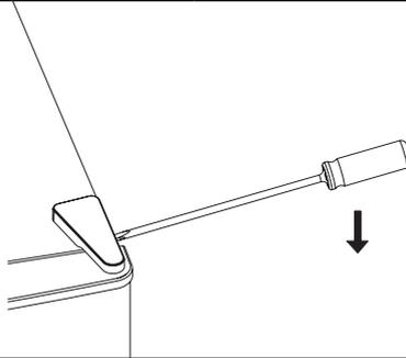
2. Unscrew the top hinge with a phillips screw driver.
