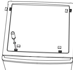
2. Unscrew top hinge and then remove upper door and place it on a soft to avoid scratch.
