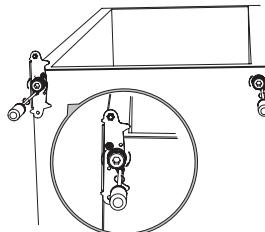
9. Make the middle hinge reverse the direction 180°C, then transfer it to the left property position. Make the middle hinge pin in the upper hole of the lower door, then tight the bolts.
