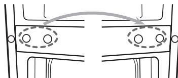
6. Unscrew bottom hinge. Then remove the adjustable feet from both side.
