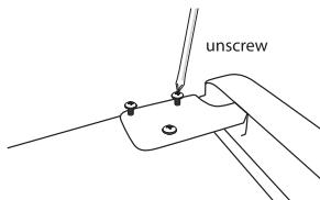
3. Remove the pin with a screwdriver and flip the hinge bracket. Then refit the pin to hinge bracket.
