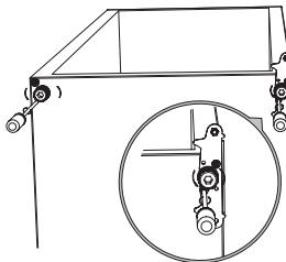
7. Unscrew and remove the bottom hinge pin, turn the bracket over and replace it.
