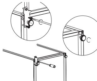
10. Place the upper door back on. Ensure the door is aligned horizontally and vertically so that the seal are closed on all sides before finally tightening the top hinge. Then inert the hinge and screw it to the top of the unit.
